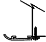
Option 11 Flat Extruded Aluminum Frame Screwed Into Plenum Lip Using Pan Head Screws on 12" Centers. Off-White Finish.
