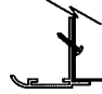
Option 12 Extruded Aluminum Frame. No Surface Screws. Fastened Thru Slot Opening. Off-White Finish.
