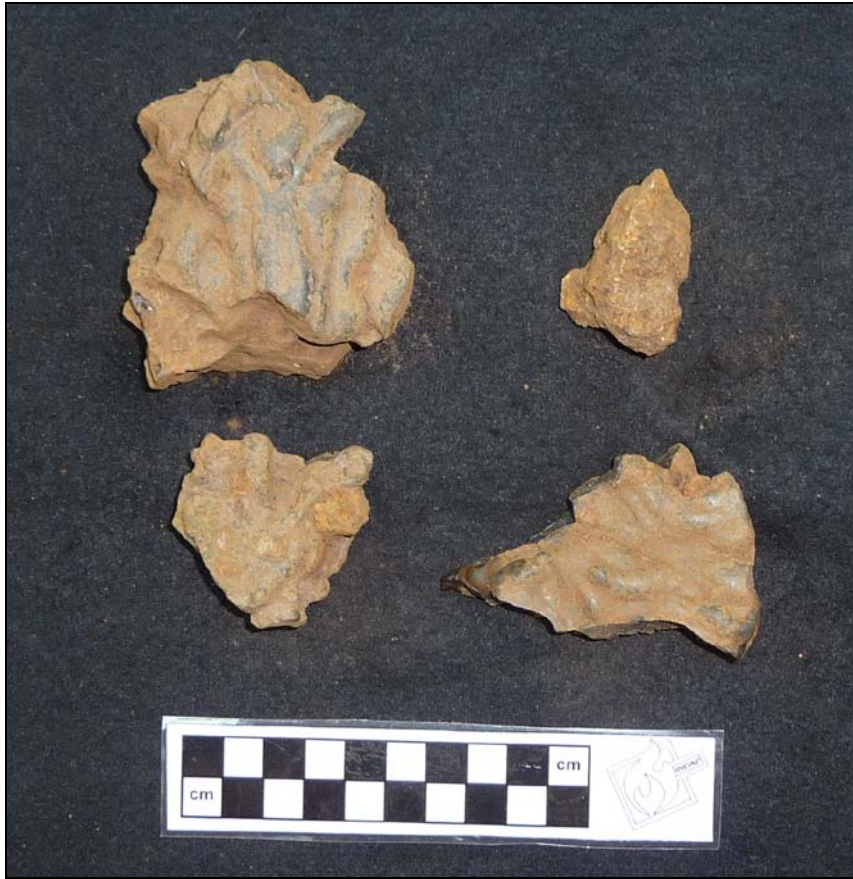
Figure 14. Examples of tap slags from Trench 1A-1002
