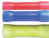
BUTT CONNECTORS - VINYL INSULATED 1700CS - RED, 22-18 GA 1800CP - BLUE, 16-14 GA 1900CP - YELLOW, 12-10 GA
