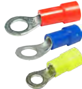
RING INSULATED CONNECTORS - #10 - VINYL INSULATED 1705CS - RED, 22-18 GA 1805CS - BLUE, 16-14 GA 1905CP - YELLOW, 12-10 GA
