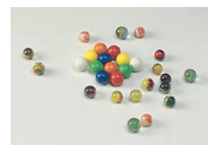
FIGURE 15-2 A mixture of magnetic marbles with nonmagnetic ones results in the separation of the two different kinds of marbles.
