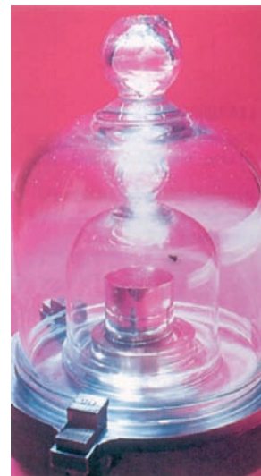
FIGURE 2-3 A duplicate of the international standard kilogram, called kilogram 20, is kept at the National Institute of Standards and Technology near Washington, DC.
