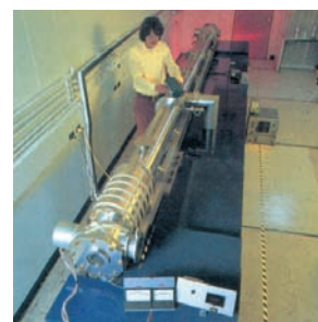
FIGURE 2-4 The standard of time, the second, is defined using a cesium clock.
