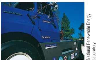
This truck is powered by liquid propane, also known as LP gas, a clean fuel with very low emissions.
