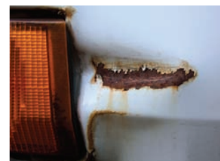
Paint will protect iron by forming a barrier to moisture and oxygen; however, a chip in the paint will result in rusting.
