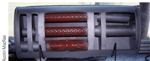
FIGURE 9-9 Cutaway of an automotive catalytic converter.
