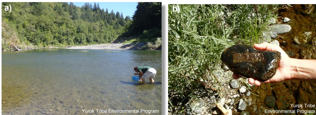
Figure 4. Photographs: (a) collecting a cobble at Trinity River near Weitchpec (TR) periphyton monitoring site, July 17, 2013, (b) a cobble with periphyton removed from everywhere except the 1-inch x 3-inch sampling area (from a different sampling site).
