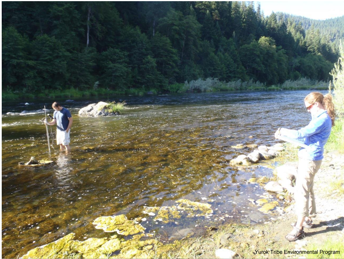
Figure 3. Photograph of field crew measuring velocity and light extinction at Klamath River below Happy Camp (HC) periphyton monitoring site, July 18, 2013.
