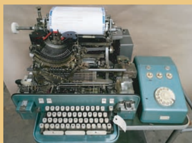
SEL-Lorenz Lo 15 open case (electromechanical page printer) (r.1967) Local line 13
