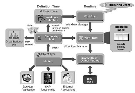
Figure 24: Workflow: Design and Sequence of Events II
