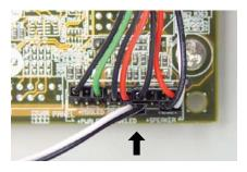
Connect the female ATX power lead from the Slot Adapter to the motherboard's power switch connection (often marked "PWRSW", "PWSW", or "PWBT").
