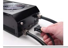
Once the hoses are connected, plug the external power cable into the cooling system.
