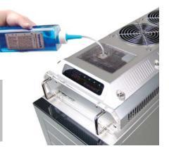
Slowly fill the system. **To maintain the product warranty, use only Koolance approved coolant.** Many alternative liquids and additives can cause permanent damage to the cooling unit (through chemical reaction, corrosion, biological growth, thermal expansion, viscosity, etc.).
