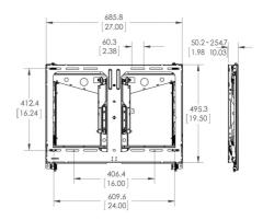
The PFW 6880 are suitable for displays weighing up to 45.5 kg / 100 lbs. with a mounting pattern of  $200 \times 200 \times 600 \times 400 \text{mm}$ .
