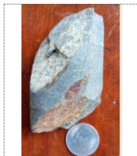
Photo 12. Dolerite intrusion in to charnockite, BH-5, depth interval 13.00-14.50m.
