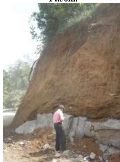
Photo. 13. Weathering Profile of Grey Colour Over Felsic Rock, road cut towards Puthumala.
