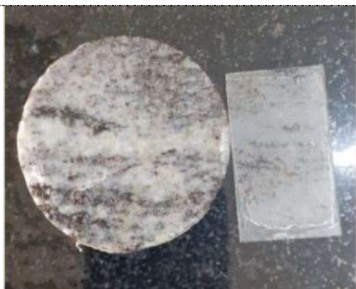
Photo 8. Core sample of Quartzo feldspathic Neosome (white), BH-8. Thin Section on the Right Side
