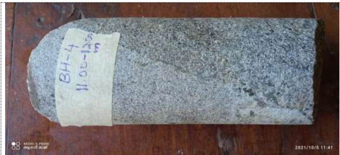
Photo 3. Greasy Patches in Charnockite from Core Sample, BH-4.
