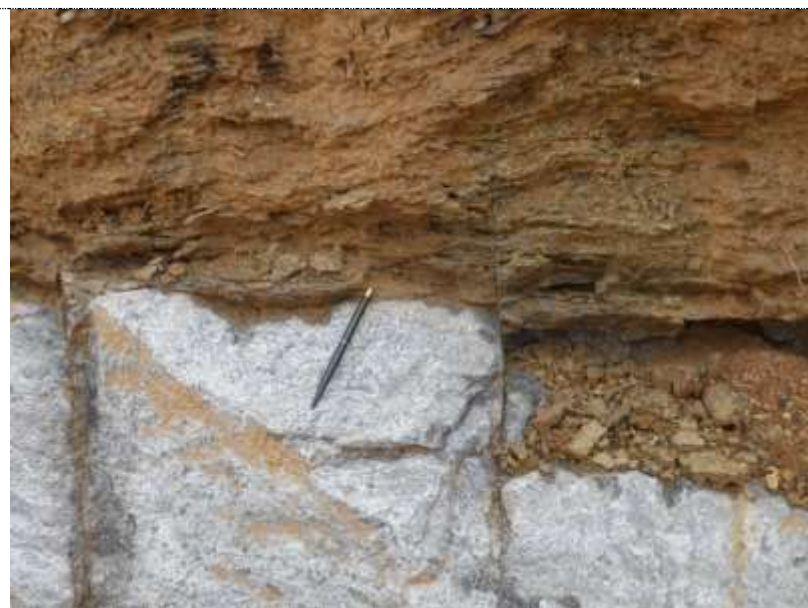
Photo 4. Charnockitic gneiss in contact with fracture, Road cut Meppadi-Chooralmala road. Also note the weathered quartzite that has been fractured (post weathering)
