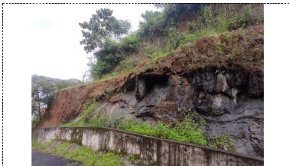
Photo 2. Massive Charnockite with Occasional Greasy Patches, Fractured . Govt. Polytechnic College Compound, Meppadi
