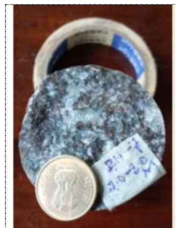
Photo 6. Large Crystals of Amphibole in Quartz-feldspar Matrix (BH-7)
