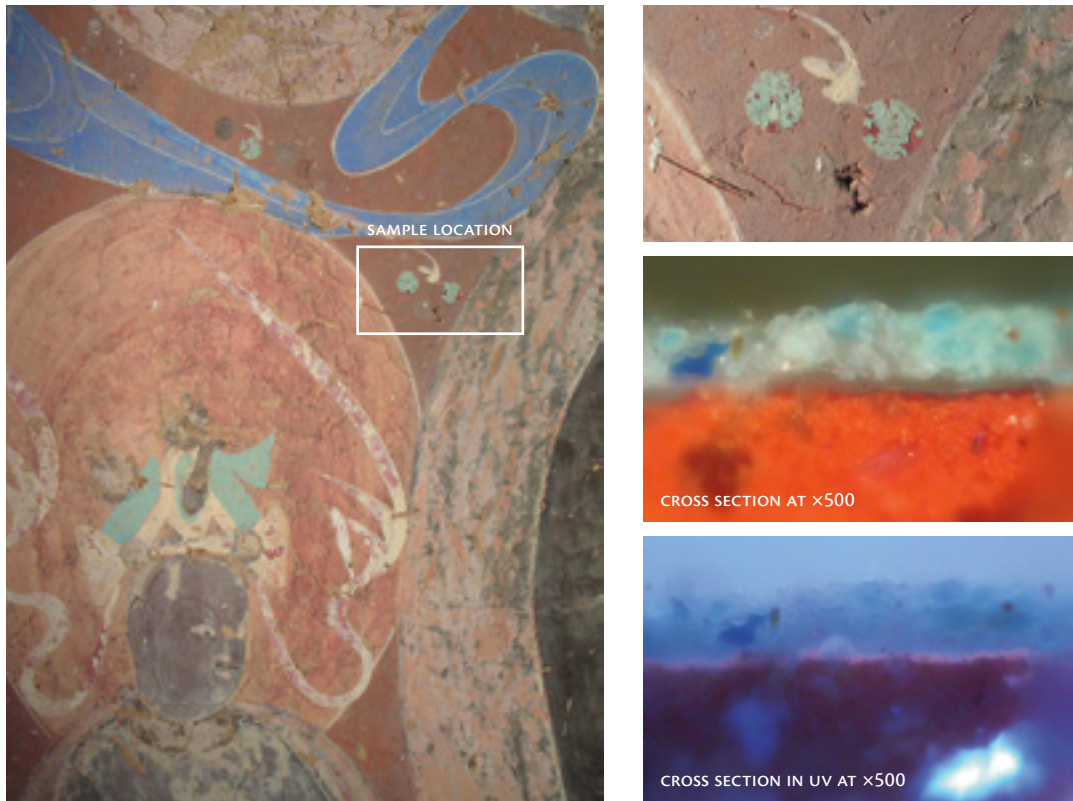
FIGURE 2 A rich crimson organic glaze applied over the iron-oxide red background survives in its unaltered state only where it has been protected by subsequent paint layers (left). A stratigraphic sample obtained from a blue detail (top right) shows a well-preserved layer of organic red beneath the blue when mounted in cross section (center right), which luminesces bright pink under UV excitation (bottom right).
