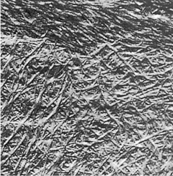
Figure 3.6. A small section of cell wall, as seen in a transmission electron microscope. The filaments are cellulose.
