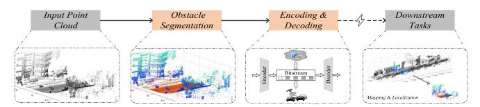
Fig. 1. Pipeline of the proposed task-driven SA-LPCC framework for autonomous vehicles. To eliminate the influence of movable objects, we develop a multimodal-based semantic segmentation scheme for LiDAR data. To reduce storage space and transmission bandwidth, we develop a plane-fitting-based method to remove spatial redundancy and investigate an unsupervised interframe network to remove temporal redundancy. Finally, we evaluate our SA-LPCC performance on some downstream tasks.
