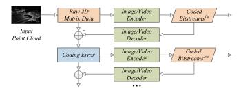
Fig. 6. Architecture for the proposed PC-HEVC method. The input LiDAR data is first converted to a 2-D matrix, quantized to 8 b, and encoded by the HEVC standard method. The coding error is calculated, and this encoding procedure is repeated until the reconstruction accuracy is met.
