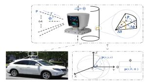
Fig. 2. Illustrations of a typical LiDAR sensor and the associated coordinate transformation.
