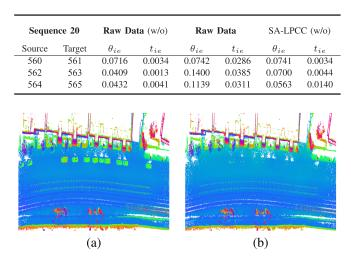
Fig. 10. Mapping results on the KITTI dataset. (a) Using the original point clouds. (b) Using the decoded point clouds with SA-LPCC. As seen, there are vehicles in the point cloud map built using raw point clouds, which may have confrontational impacts when used for localization or navigation. Using our SA-LPCC, the "noise" information is effectively removed, and a clean map is obtained.
