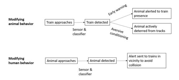
Figure 5. Conceptual mechanism underlying technology-based mitigation of wildlife-train collisions.
