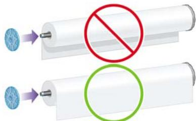
Ensure there is no space between the roll and the fixed stop at the right-hand end of the spindle.
