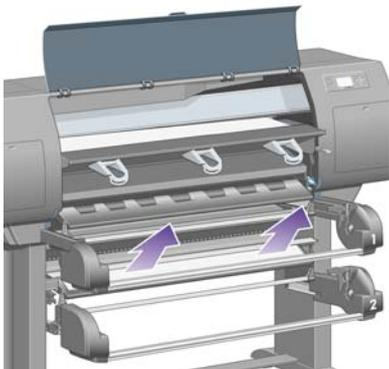
11. Carefully remove any paper that you can lift up and out from the top of the printer.
