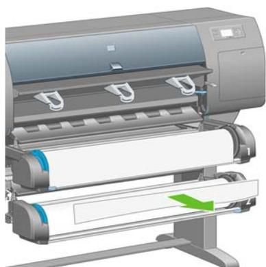
6. Rotate the spindle backwards to move the paper edge out of the way.
