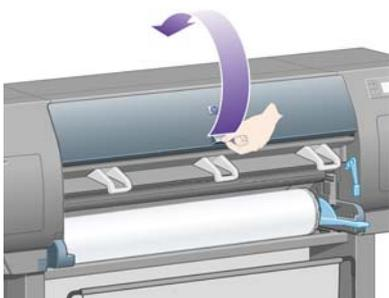
3. Try to move the printhead carriage out of the way.
