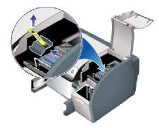
Peel off the label prior to removing the stopper latch.
