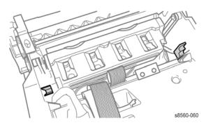
**Figure 9 Printhead Cradle Notch Location**
