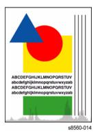
Figure 1 Example of Oil Streaks on Output
