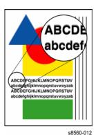
Figure 1 Example of Poor Text Resolution on Output
