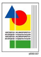
Figure 1 Example of Scratches on Output
