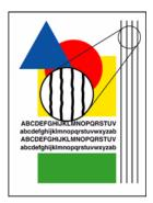
Figure 1 Example of Wavy Vertical Lines on Output
