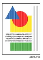
Figure 1 Example of Pinstripes on Output
