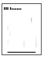
Figure 1 Example of Smudged or Smeared Output
