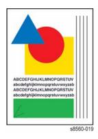
Figure 1 Example of Wrinkled Output
