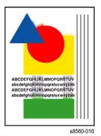
Figure 1 Example of Ink Smears on Output
