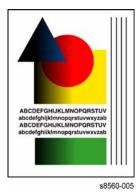
Figure 1 Example of Uneven or Incorrect Color Output
