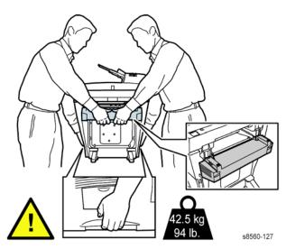
Figure 2 System Lifting Technique
