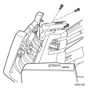
**Figure 1 DADF Front Cover Fasteners**
