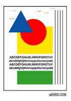
Figure 1 Example of Latent Image on Output
