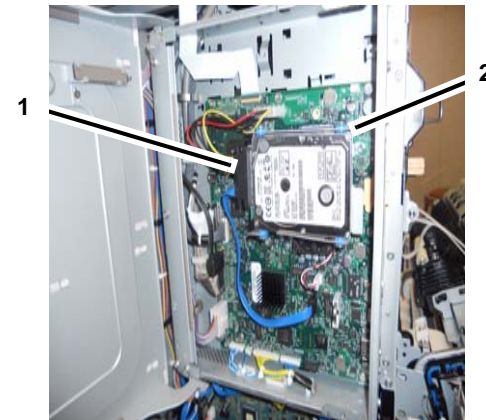
Figure 1 HDD Removal Preparation
