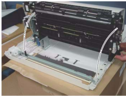
Figure 3 Align the Positioning Pin
