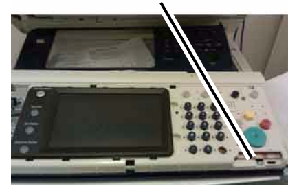
Figure 5 UI Lower Cover Removal
