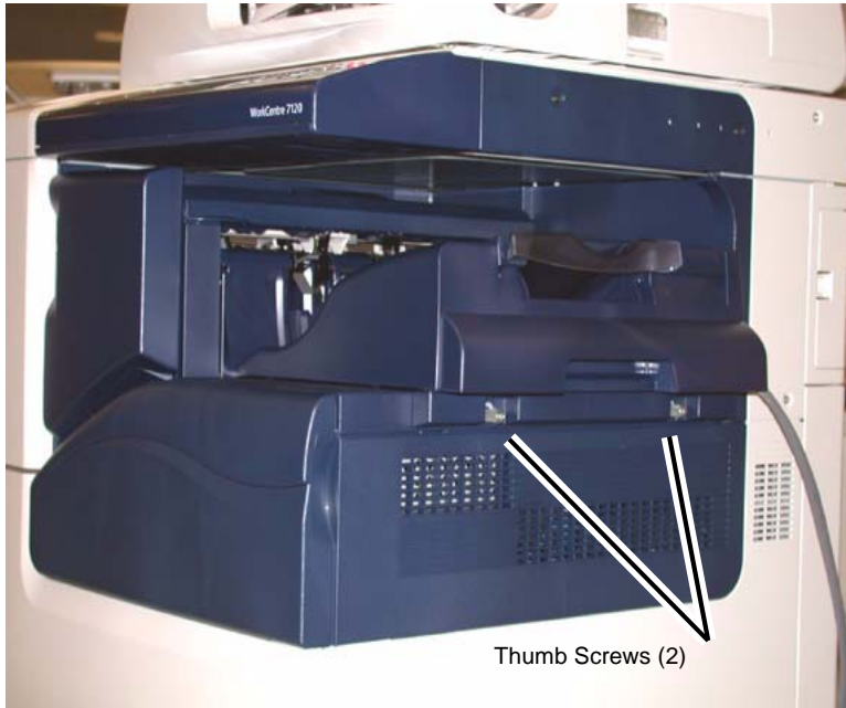
Figure 3 Loosen the Thumb Screws
