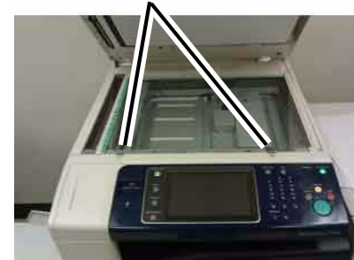
Figure 1 Control Panel Screws
