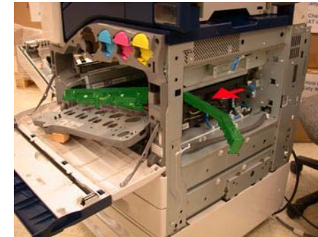
Figure 4 Repositioning the High Voltage Conductor Housing Assy
