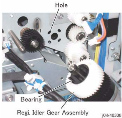
Figure 2 Reg Idler Gear Assy Alignment
