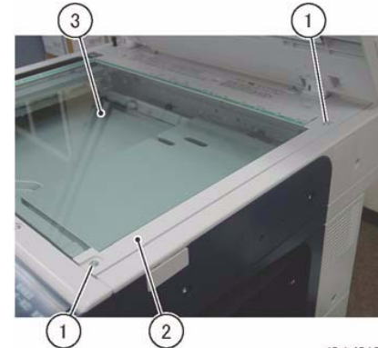
Figure 1 Platen Glass Removal
