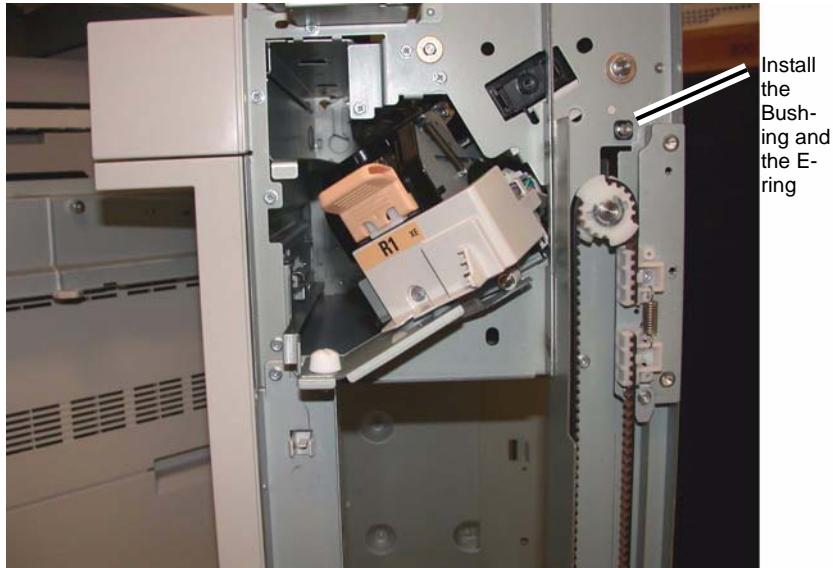
Figure 16 Installing the Bushing and E-ring
