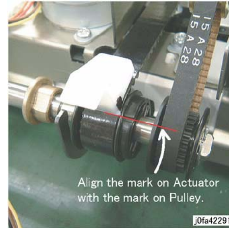
Figure 6 Align Eject Belt
