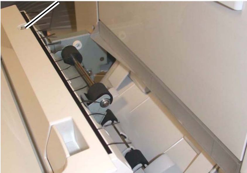
Figure 6 Installing the Retaining Screw
