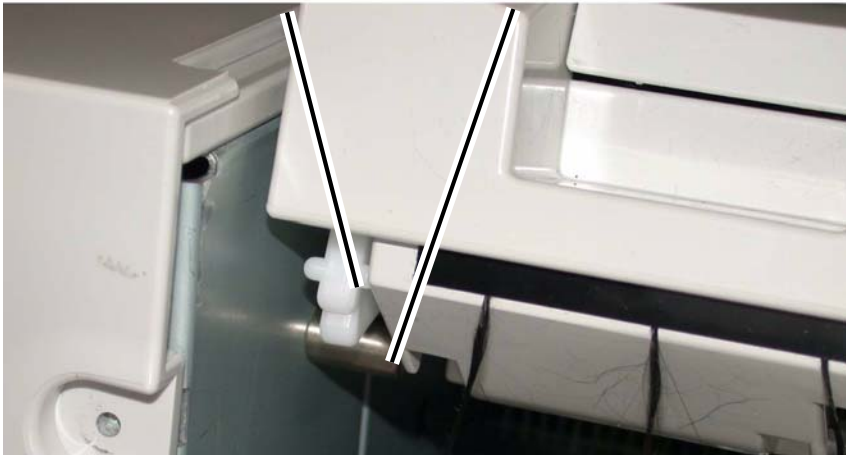
Figure 5 Positioning the Latch Hook and Latch Pin
