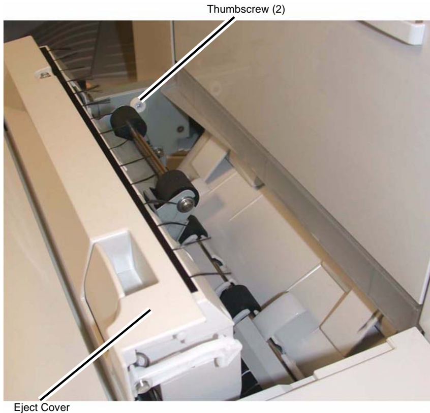
Figure 1 Eject Cover and Thumbscrew
