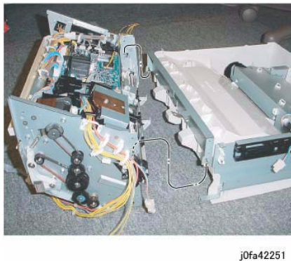
Figure 5 Installing the Stacker Tray Assembly
