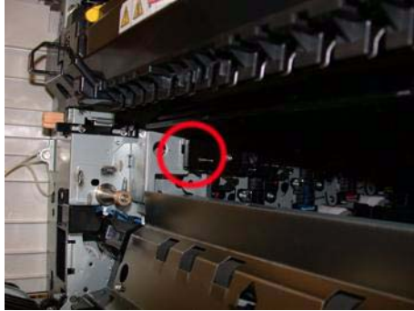
Figure 6 High Voltage Conductor Housing Assembly Tab
