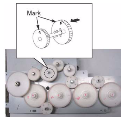
Figure 4 Triangular Marks Alignment
