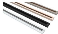
K5-3 Single Circuit/Two Circuit Track Single Circuit Track is rated for 2400W Features 12-gauge copper conductors and a separate ground conductor. Two circuit track includes 12-gauge copper conductors and features a double load capacity at 4800W max. Single/Two Circuit Track is available in white, black and satin nickel finishes, and in 4, 6, and 8-foot sizes, and can also be field cut to your preference.
