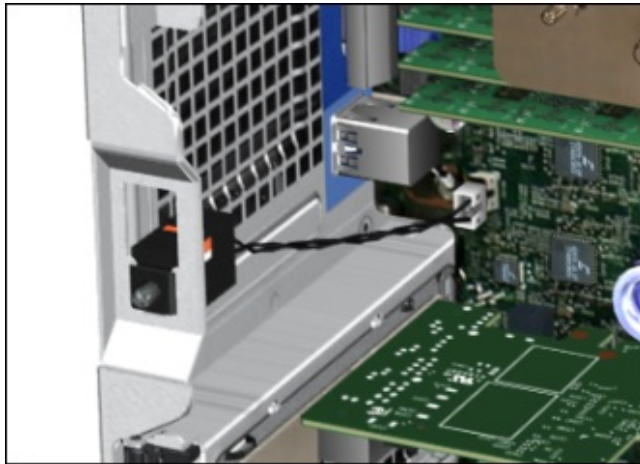
Figure 9. Chassis intrusion switch
