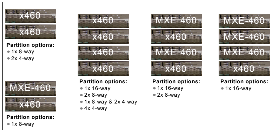
Figure 2-3 Supported partitioning for 2-node and 4-node complexes
