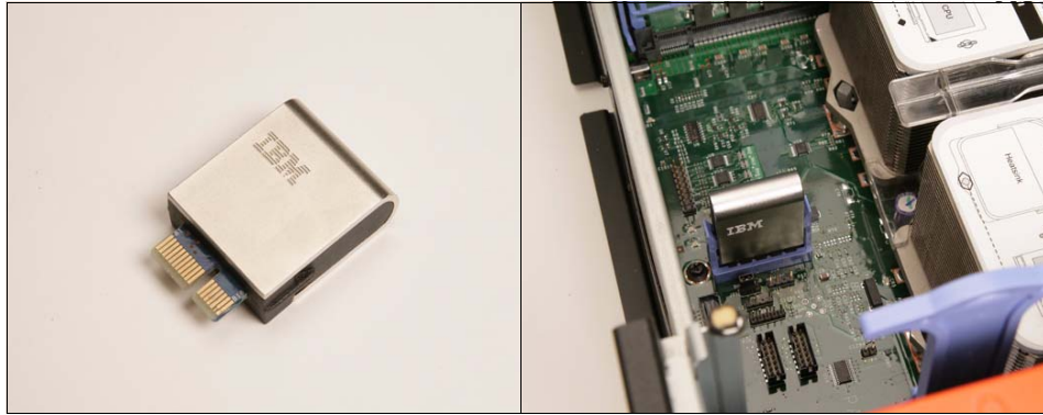
Figure 4-5 ScaleXpander key (left); ScaleXpander key installed on processor board near the front of the x3950 M2 (right)
