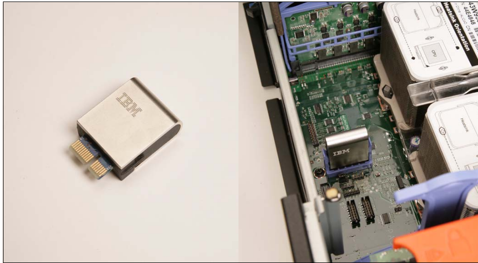
Figure 1-5 ScaleXpander chip (left); ScaleXpander chip installed on processor board near the front panel of the x3950 M2 (right)
