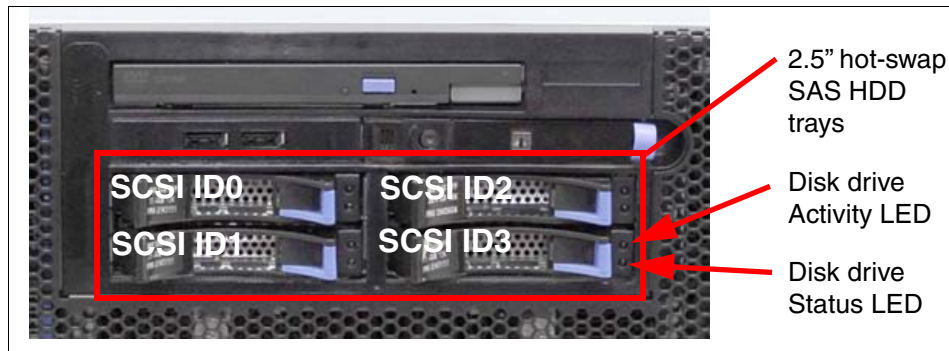
Figure 3-20 Media hood: hard disk drive bays
