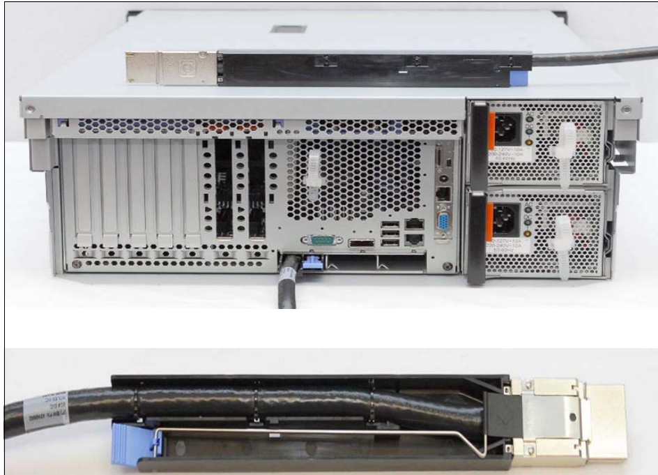
Figure 1-6 Scalability cable (top); cable installed in SMP Expansion Port 1 (bottom)
