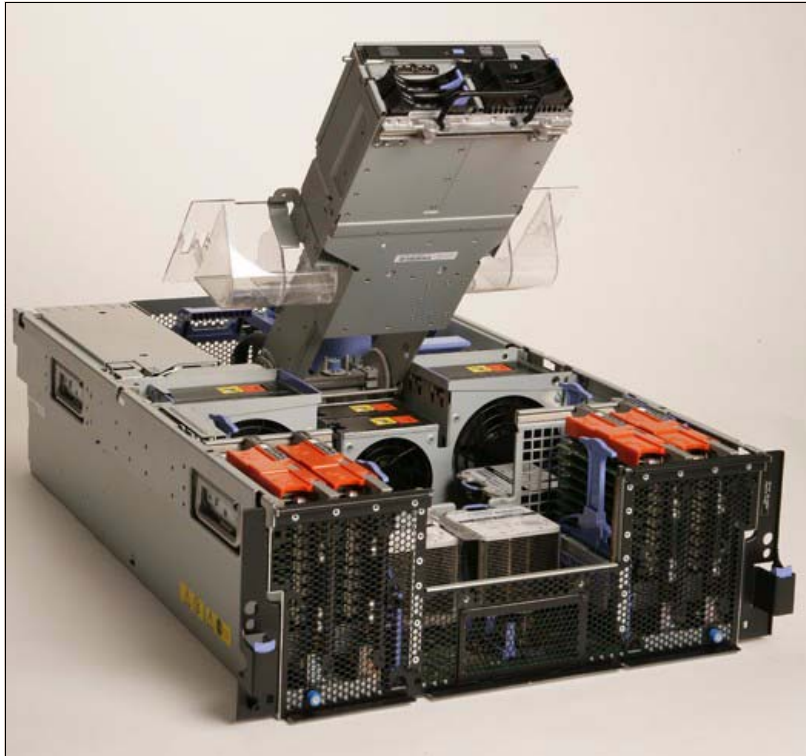
Figure 3-2 Media hood opened to access the processors
