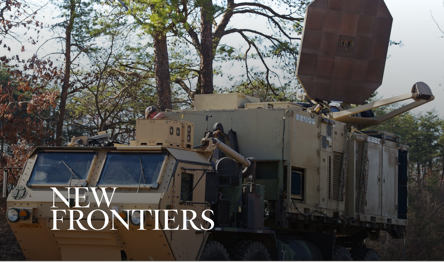
"A US MARINE CORPS TRUCK IS SEEN CARRYING A PALLETIZED VERSION OF THE ACTIVE DENIAL SYSTEM, MARCH 9TH, 2012, AT THE US MARINE CORPS BASE QUANTICO, VIRGINIA." PAUL J. RICHARDS | AFP/GETTY IMAGES
