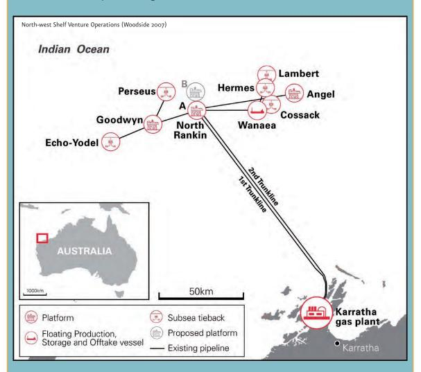
The North West Shelf Venture has three offshore facilities: North Rankin A, which is one of the world's largest gas producing platforms, Goodwyn A, which produces large volumes of gas and condensate, and Cossack Pioneer floating production, storage and off-take facility, which produces oil. The project also produces crude oil from the Cossack, Wanaea, Lambert and Hermes oil and gas fields.
