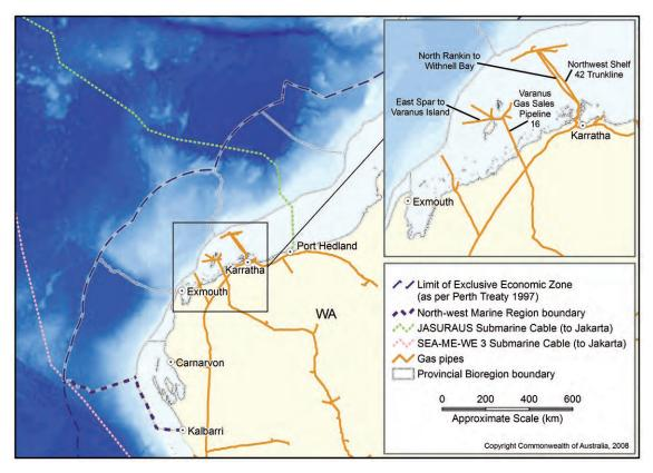
hard limestone. The cable is buried from the coast to 100 km offshore to protect it from damage and breakage in shallower water. The JASURAUS Cable was laid in 1997 has a technical life of 25 years.
