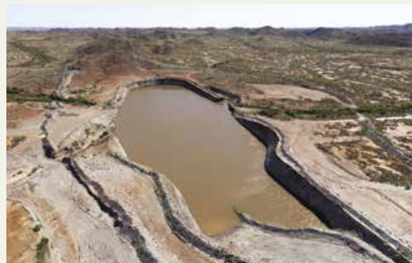
Iron ore mining requires the creation of huge waste dumps (shown below at Mount Tom Price Mine) and the disposal of large volumes of water when mining drops below the watertable. Water from Hope Downs Mine is discharged into Weeli Wolli Creek (top left, photographed in about 2003). And after mining ends, unless the mining pit is filled in, it becomes a pit lake (top right, at Woodie Woodie). There are about 100 pit lakes in the Pilbara, with the potential for hundreds more. Images: Josef Furulyas Snr (top left), Krystle Wright (top right & bottom)
