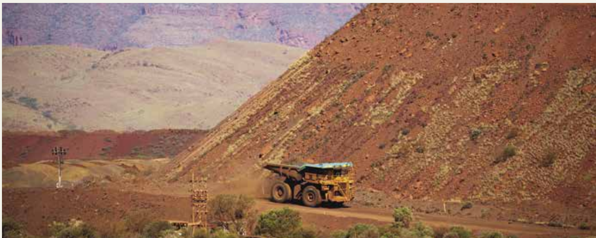
Iron ore mining requires the creation of huge waste dumps (shown below at Mount Tom Price Mine) and the disposal of large volumes of water when mining drops below the watertable. Water from Hope Downs Mine is discharged into Weeli Wolli Creek (top left, photographed in about 2003). And after mining ends, unless the mining pit is filled in, it becomes a pit lake (top right, at Woodie Woodie). There are about 100 pit lakes in the Pilbara, with the potential for hundreds more. Images: Josef Furulyas Snr (top left), Krystle Wright (top right & bottom)
