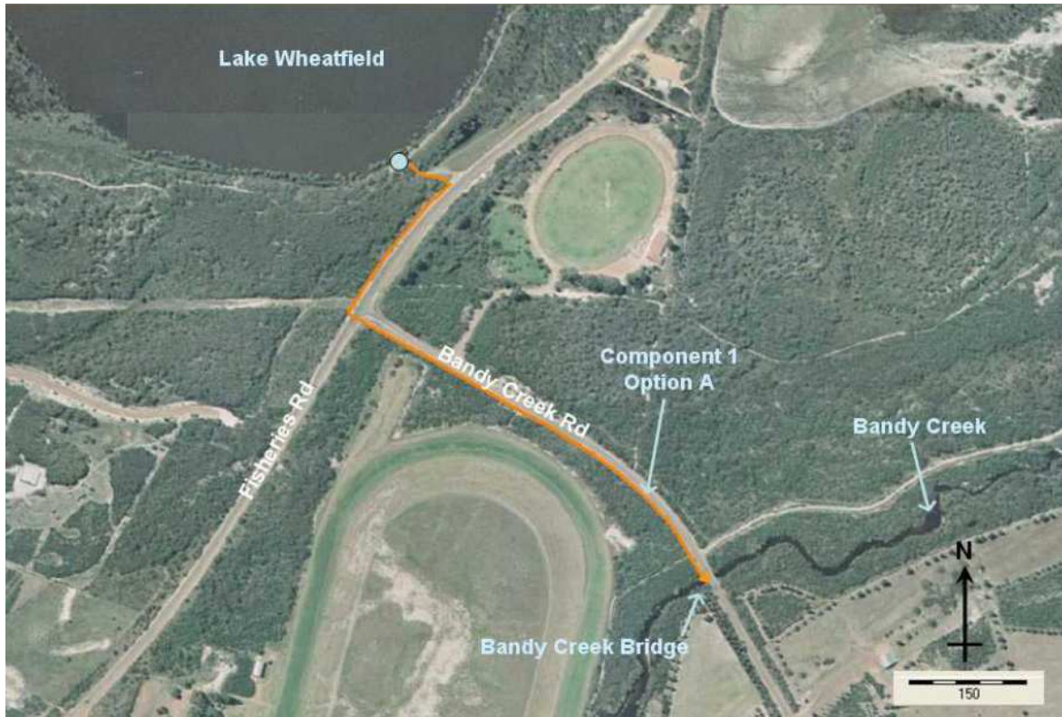
Figure 3. Component 1 Option A – Siphon Pipe Alignment
