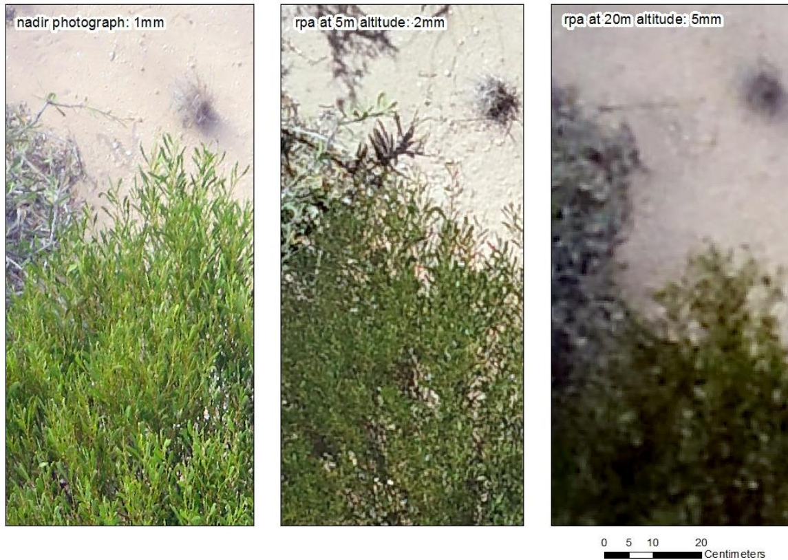
Figure 1: A comparison of imagery from nadir photography (1 mm resolution), RPA at 5 m altitude (2 mm) and RPA at 20 m altitude (5 mm).
