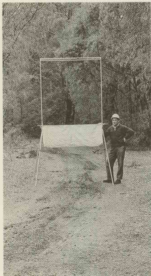
Plate 17▲ Collapsible bat trap constructed after the design of Tiedemann and Woodside (1978).
