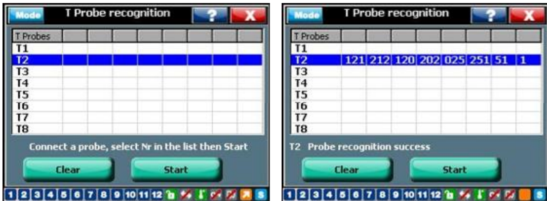
Figure 45: Temperature probe auto recognition
