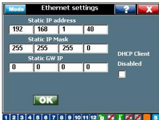
Figure 56: RVT TCP/IP protocol setting
