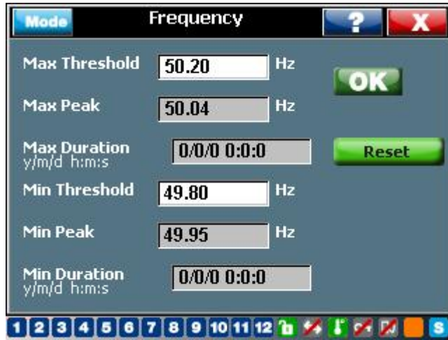
Figure 25: Event logging threshold setting - Frequency
