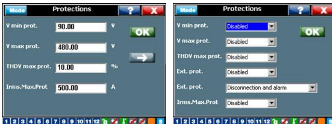
Figure 40: RVT protection settings
