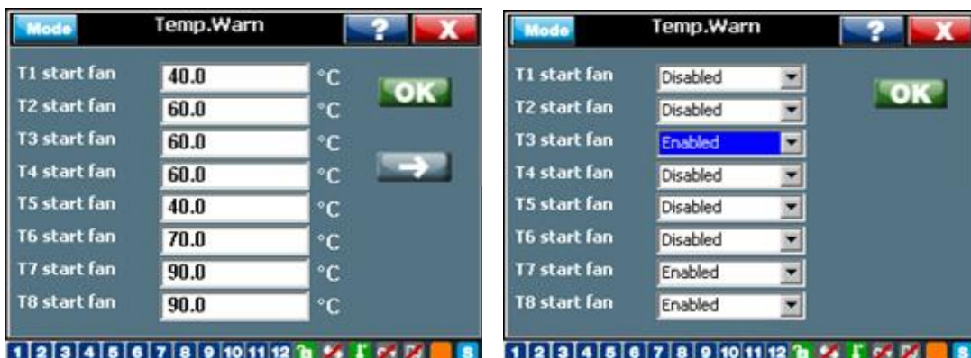
Figure 43: RVT temperature warning settings
