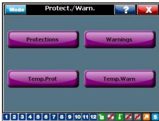
Figure 39: RVT protections and warning settings
