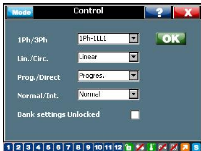
Figure 34: RVT bank settings protection: not protected
