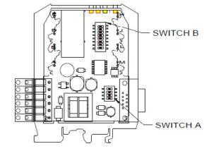
SWITCH A: used for hardware configuration of RS485
