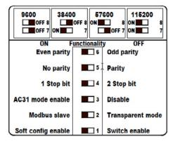
**1:** Soft / switch configuration selection. When this switch is set to the on position switch configuration is ignored, and the system is configured using the software. When it is set to the off position, switch configuration is valid.
