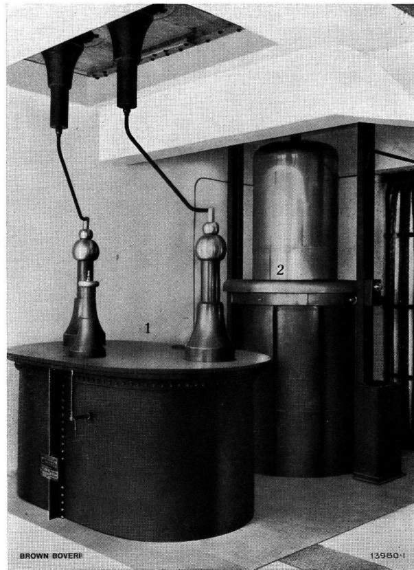
Fig. 11. — Part of the cellar below the dark room. 1. Testing transformer for 225 kV. 2. Air-gap condenser with variable capacity.
