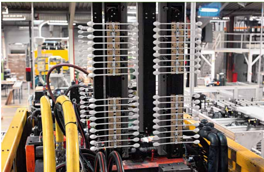
IRB 6650 taking spoons out of an injection molding machine at deSter in Belgium
