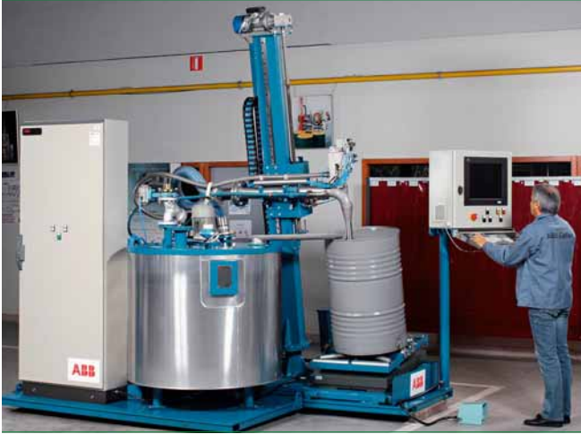
7 A drum decanting unit (DDU)
