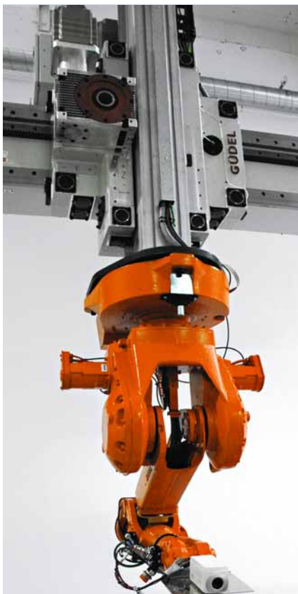
6 An ABB robot equipped for visual inspection mounted on flexible gantry crane
