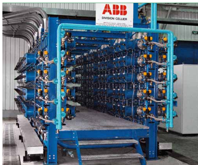
5 A piggable manifold installed in the Sinopec plant (China)
