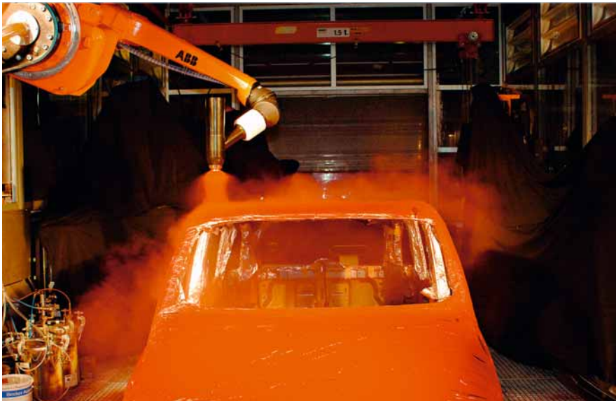
2 ABB robot spray painting in an automotive production facility
