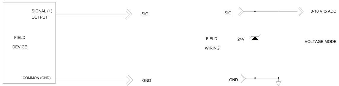
TYPICAL VOLTAGE INPUT FIELD WIRING
