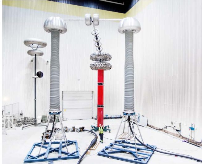
Figure 6: Type testing of the 525 kV extruded HVDC cable system.
