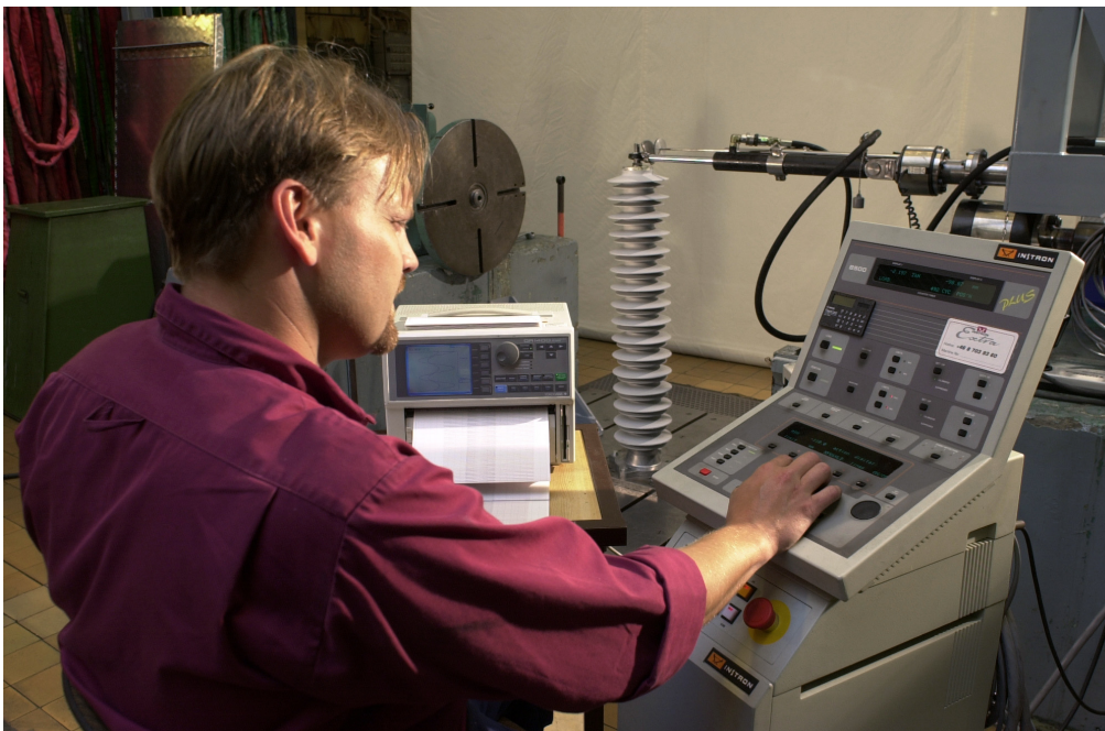
Mechanical test of silicone-housed arrester PEXLIM P.
