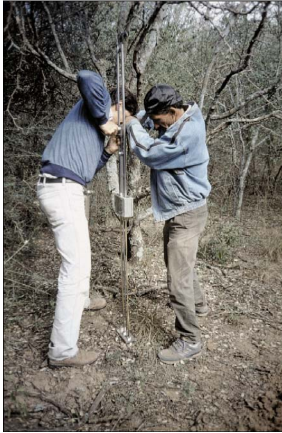
Photo 32. Stiboka penetrometer used for determining and recording soil resistance to penetration. (AZ)
