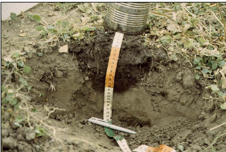
Photo 31. Wetted soil cross-section in a field reclaimed before 1970. The soil is friable till 20 cm depth, but compact underneath. Burruyacú area (Lobo farm). (EB)
