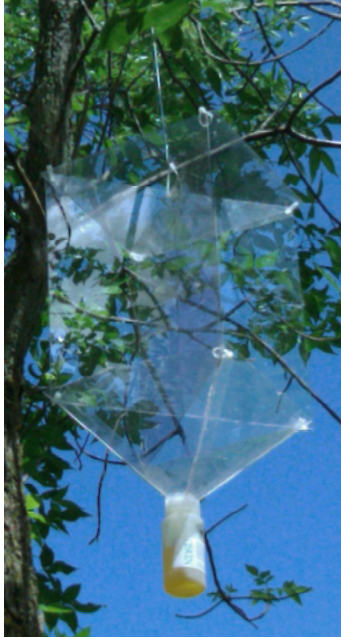
Figure 7. Free-hanging window pane flight intercept trap (FIT). (Photograph courtesy of Dr. Gerald Fauske).
