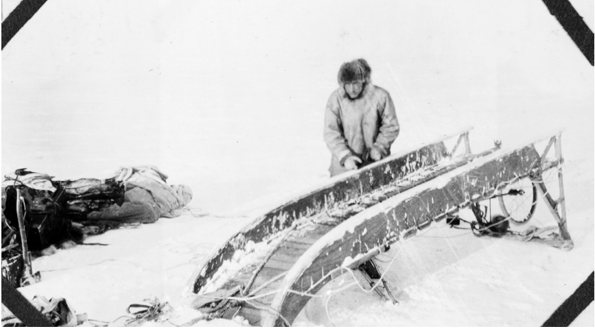
Runner made smooth with plane before final coating of ice, Pullen Point, Alaska, 1927 (Photo: AEP, LAC, e010933871)
