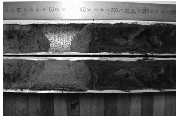
Figure 13.9 Core taken from below the limits of excavation, Square S. Note distinctive break (at c.75cm below ground surface) between coarse light yellow sands and dark organic muds.
