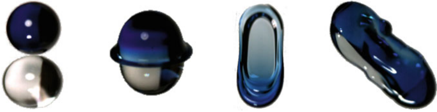
Fig. 5 Results from an experimental study of the wetting behaviour reported in [41]. This study was performed in a cooperation of sub-projects A7, B1 and C4 together with D. Baumgartner and C. Planchette from TU Graz. 73% Glycerol- water solution (G73) (transparent) colliding with an other droplet (blue) of Bromonaphtalene (B) as a partially wetting liquid or Silicon Oil M5 (SOM5) as a fully wetting liquid. From left to right: G73 + B just before collision; G73 + SOM5 rim formation; G73 + B disc formation; G73 + B retraction of the contact line after collision (dewetting). The collisions finally show separation into two or multiple droplets
