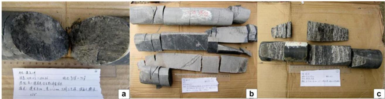
**Fig. 4.75** Tectonic seam features of Longmaxi Formation in Southern Sichuan Basin and its periphery **a** oblique crack, scratch developed, DY1; **b** high-angle fracture, unfilled, DY1; **c** high-angle fracture, calcite filled, DY1
