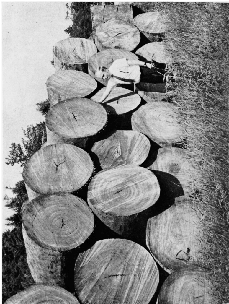
FIGURE 4. A load of Rubinga which has been shipped in by rail in twenty-foot lengths and was subsequently bucked into short lengths. End checking indicates that a certain amount of waste upon resawing can be expected. The wood will primarily be used for knife handles.
