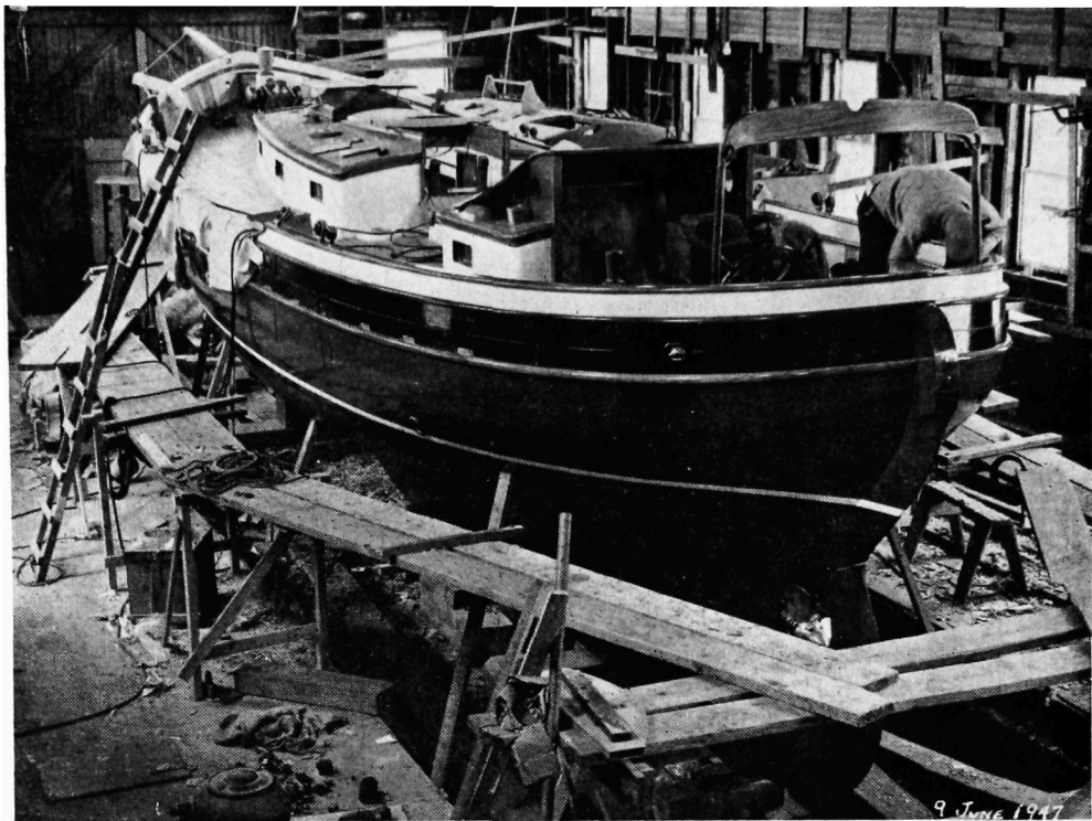
FIGURE 1. Many boats such as this one are constructed each year along the Maine coast and require outstanding craftsmanship. Often these boats utilize such woods as Burma teak for decking and Philippine mahogany for planking, as well as a number of other foreign and native woods.
