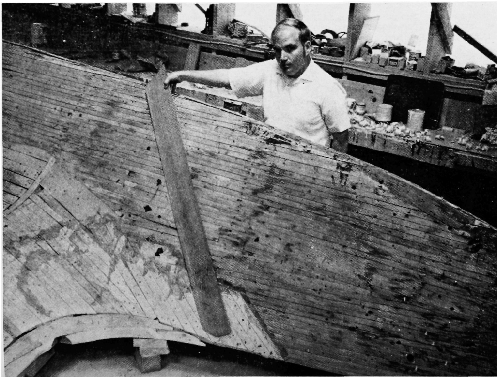
FIGURE 2. A strip of one-eighth inch African mahogany veneer laid over part of the form for construction of a Trimaran. The hull is constructed by covering the form with three layers of African mahogany, each layer being oriented in a different direction.
