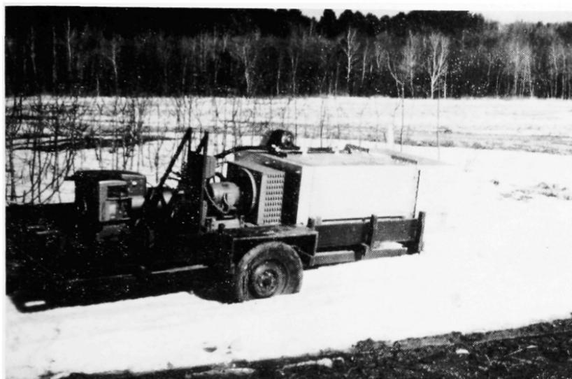
FIGURE 3A. The trailer containing the entire freezing equipment.
