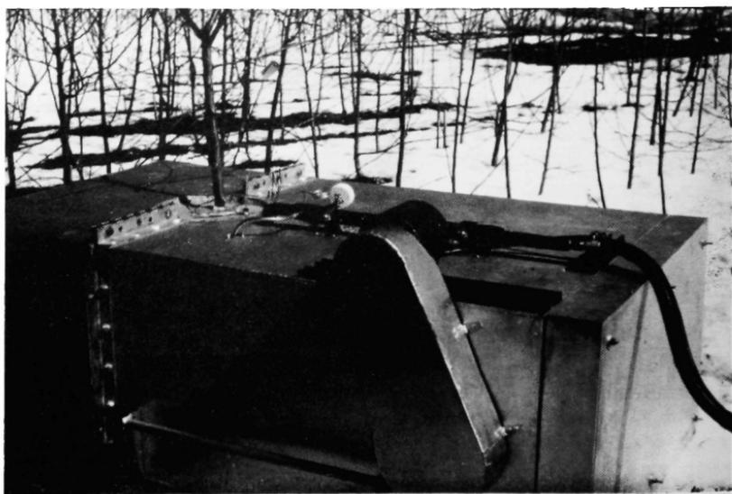
FIGURE 3C. The freezing cabinet in operation around a tree.
