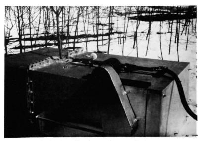
FIGURE 3C. The freezing cabinet in operation around a tree.
