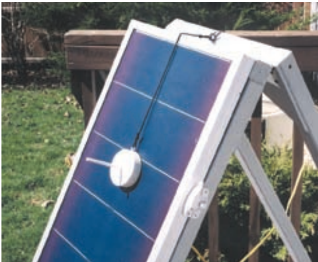
A gnomon can be temporarily used to orient PV panels. When the shadow disappears, the panel is pointing directly at the sun.
