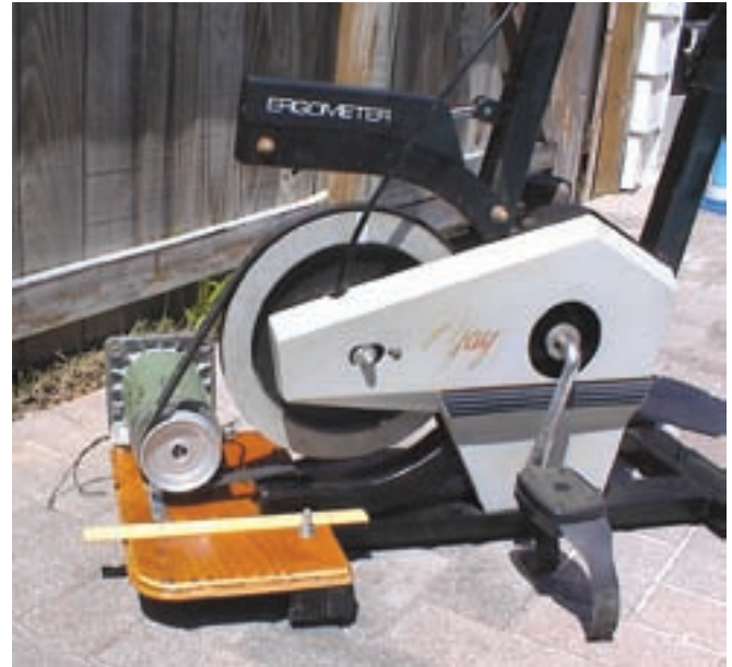
The belt-driven PM motor is mounted on a plywood platform.
