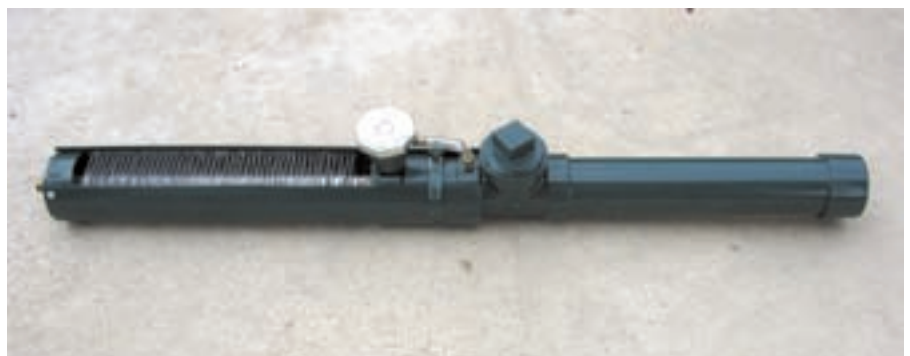
A TPFRS unit showing the radiator on the left, automobile radiator cap in the middle, and the overflow reservoir on the right.
