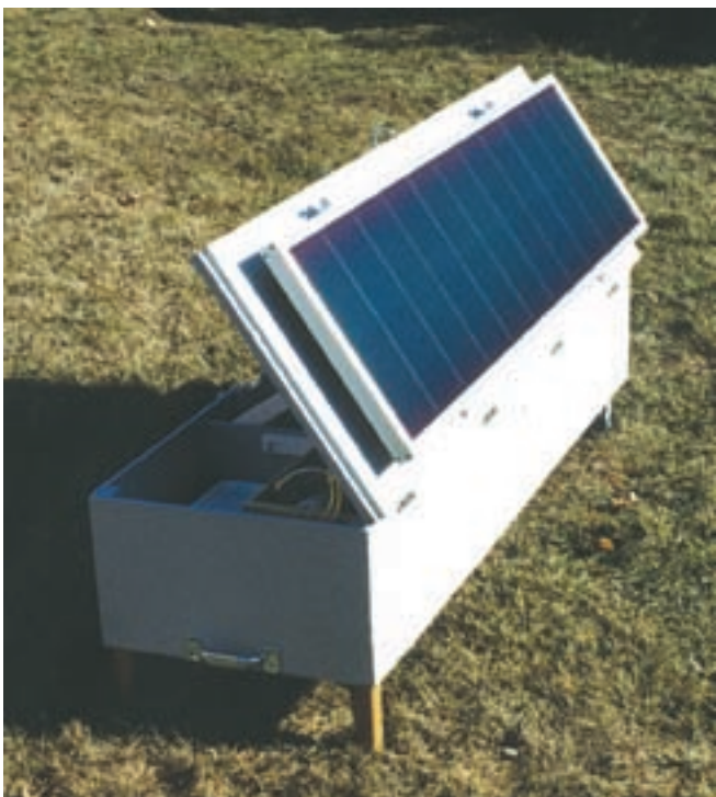
The box's hinged lid allows the PV panel to be tilted for maximum solar exposure.
