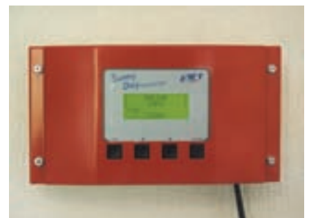
An SMA Sunny Boy Control Light system monitors performance of both inverters in the comfort of the house.
