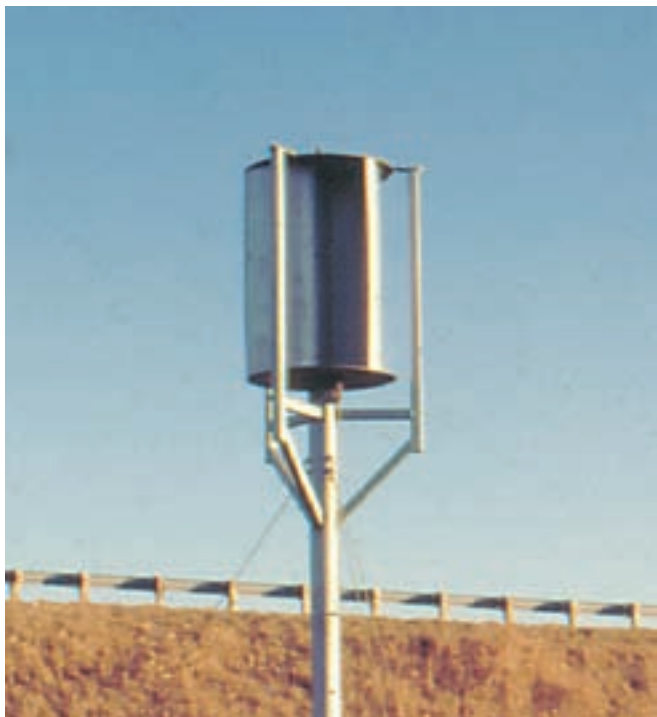
This small Savonius rotor was formed from stainless steel. Metal covers the whole swept area.
