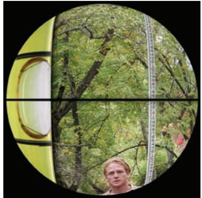
View through the sight level—Anna measured 7 feet 4 inches on the leveling rod. By subtracting the height of her eye, she determined the head for this section to be 1 foot 8 inches.
