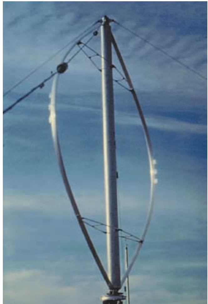
The Darrieus pictured here is a small utility-scale machine. Note the extruded aluminum blades and the guy wires, which are typical for a Darrieus.
