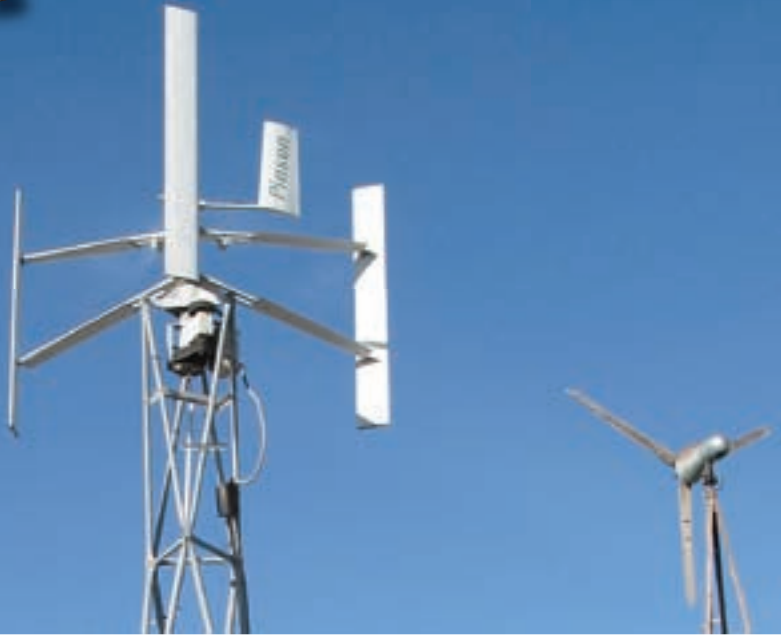
A Pinson vertical axis wind turbine (VAWT) in front of a Winpower horizontal axis wind turbine (HAWT). This Pinson turbine is an H-Rotor derivative. It features pitch adjustment for improved performance.
