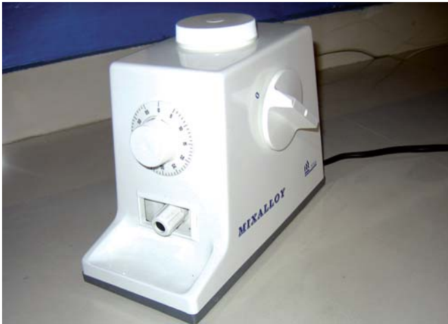
Fig. 9.6: Amalgamator used for mechanical trituration
