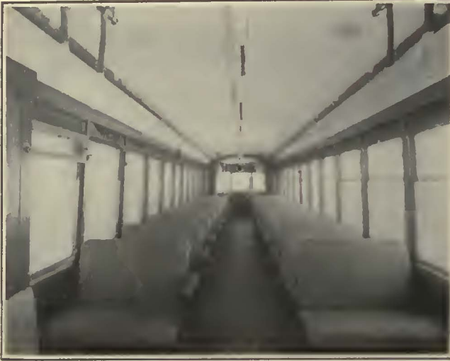
An Interior View of the New Interurban Car of the York Railways, Showing the Linoleum Floor Covering and Arm Rests
