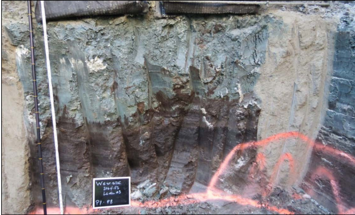
Figure 16. Level 3: clay with gasoline (blue-grey) and asphalt contamination (brown-black)
