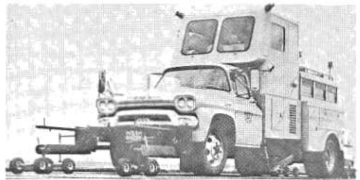
Figure 15. A photo of the Michigan Profilograph unit modeled after a California design.
