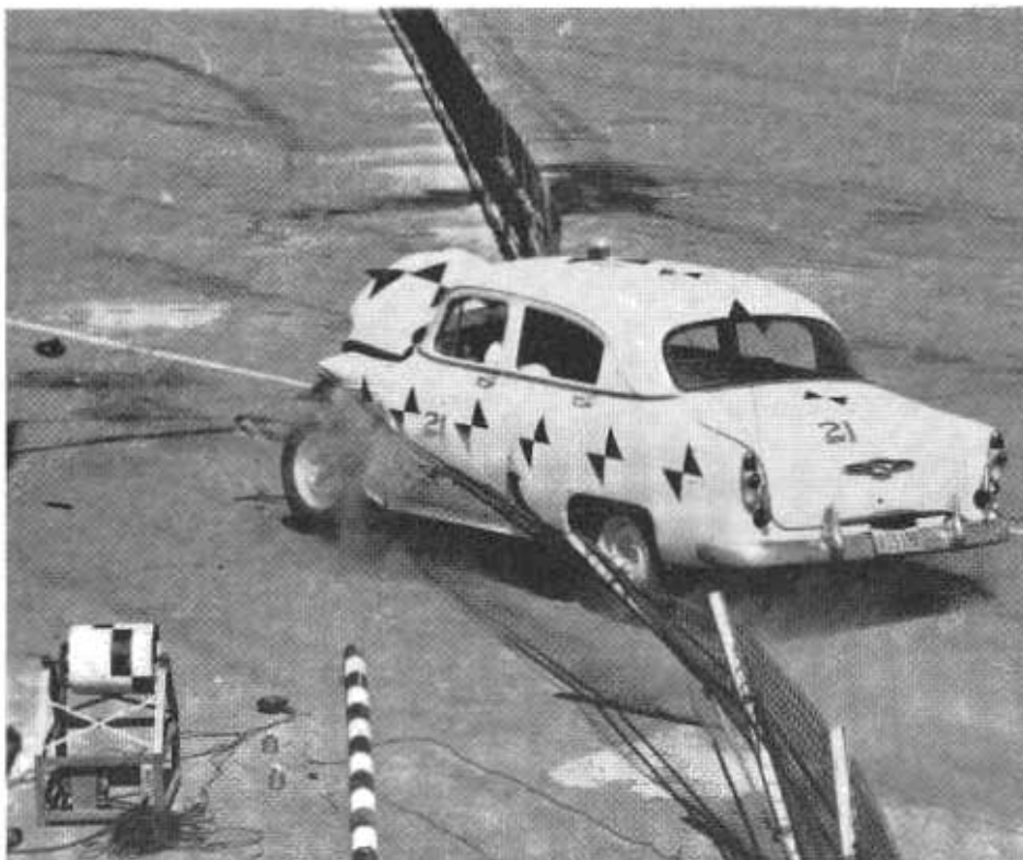
A series of impact tests was conducted in 1959 in connection with continuing research into the possible use of barriers in the center strip on freeways. A fence-cable barrier, shown as it successfully halts a radio-controlled sedan going 60 miles an hour, was one of the new barrier designs found to be most effective.
