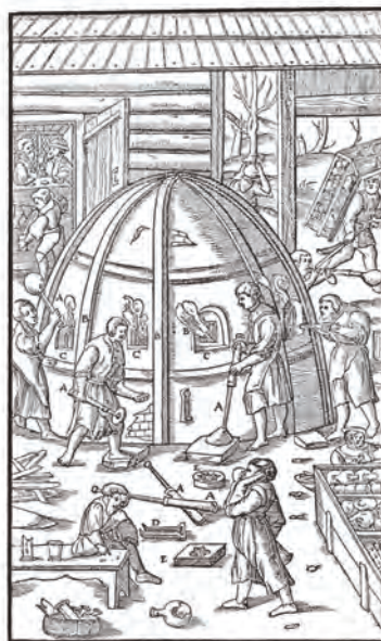
A—BLOWPIPE. B—LITTLE WINDOW. C—MAGNET. D—FURNACE. E—SHOCK OF BRASS BY WHICH THE GLASS IS PRESSED.
