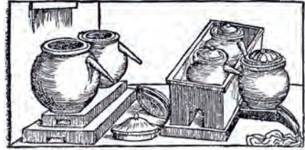
Fig. 7.27 Vanoccio Biringuccio, Tubulated vessels for the extraction of sulphur by distillation , from Pirotechnia (Venice, 1540).
