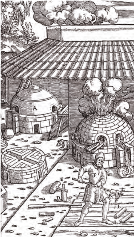
Fig. 8.6 Georgius Agricola, examples of cupelling furnaces, from De Re Metallica (Basel, 1556). Reprinted in Agricola & Hoover, 1950, p. 481.
